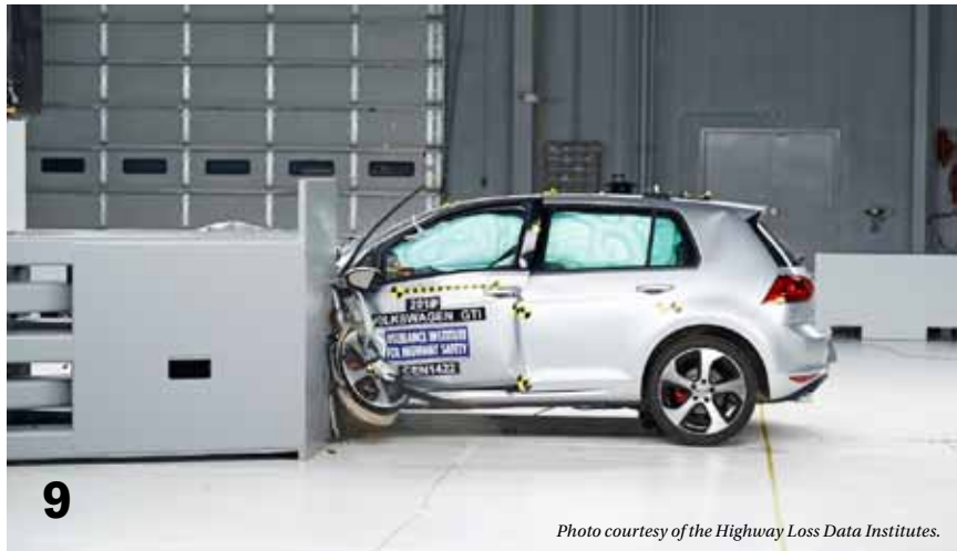
(6) Prepping 2015 VW GTI for a small overlap front test. (7) The central barrier test area. (8) The long hallway to get cars up to speed. (9) The moment of maximum deformation is shown. This vehicle did well on the small overlap front test and Volkswagen was very pleased, according to Hazelbaker.
